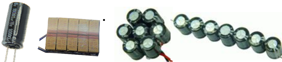
Elko Tantal-Paket 5000 \mu\text{F} Goldcap-Module mit 7 Goldcaps (7 x 1F in Serie, also 140000 F - 17,5 V)
